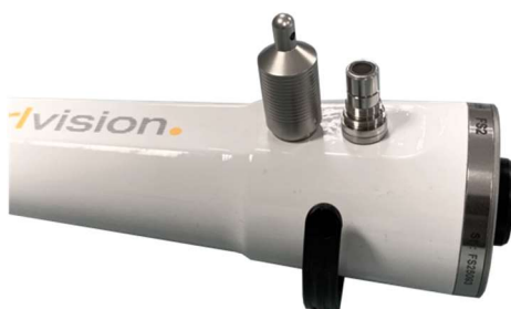
Figure 6: Valve cover cap fitted
