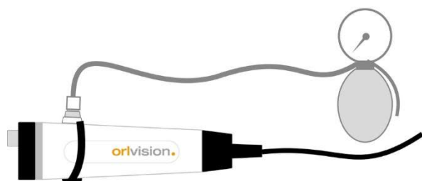
Figure: 10 Leak Tester connection
